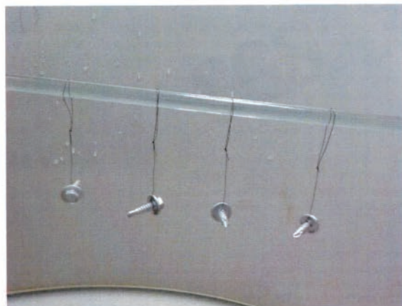
Fig. 2 : Method of Supporting specimens
