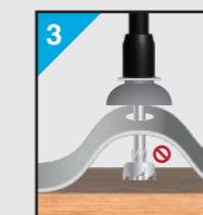
The Expansion Hole Cutter works in combination with the Depth Stop Knurls, and prevents overdriving of the screw after touching the purflin.
