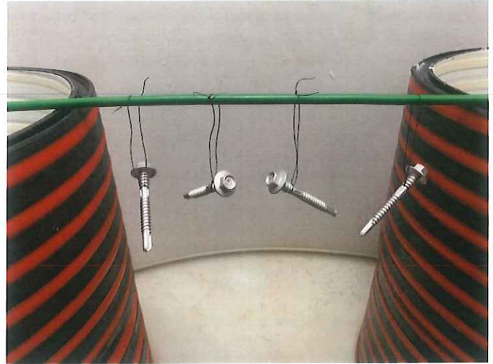
Fig. 2 : Method of supporting specimens
