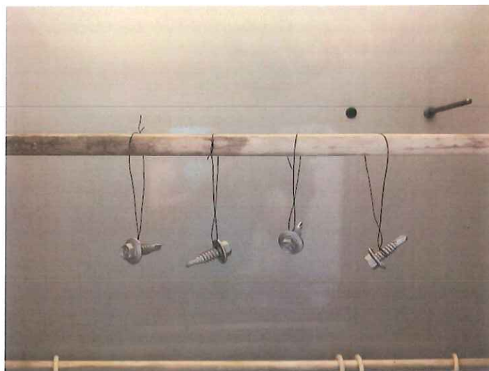
Fig. 2 : Method of supporting specimens
