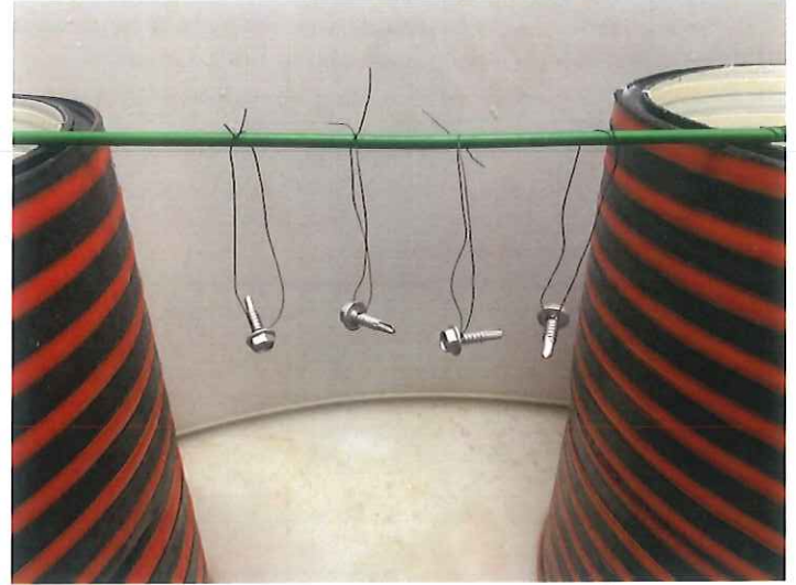
Fig. 2 : Method of supporting specimens
